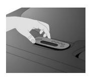
With an scraper tool, gently clean the surface of installation of the new keypad, finish the job with an alcohol saturated paper towel to remove any unwanted residue left over from the old keypad.
