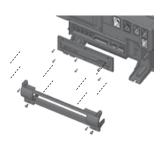
A watertight panel protects the heater and probe connectors. Removing the panel gives access to in.flo dry-fire protection and hi-limit/regulation probe connectors, line 1, line 2 and ground power input cables connection ports.
