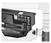
Secure the keypad in place. Insure that its adhesive strip is properly glued by pressing evenly with your finger over the entire surface.
